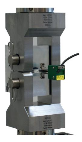
We are offering the fully range of different sizes with imperial as well as metric dimensions made from different materials for different test temperatures. All Clevis Grips are made with D-shaped pinhole and are supplied with pins and spring retainers. All necessary attachments for the test systems and pre-loading fittings are also be provided.
