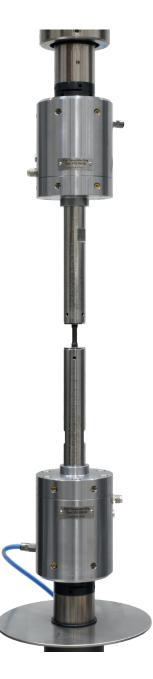
The reverse rated grip extension with inside pushrod for specimen preloading and the exchangeable specimen adapters extend into the heated zone of the furnace. These pars are made of high-temperature super alloys with high strengths at high temperature.
