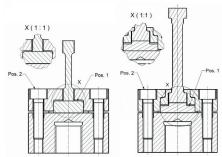
The TF Grips are available for forces up to 500 kN for ambient testing or as version for the use inside the environmental chamber.
