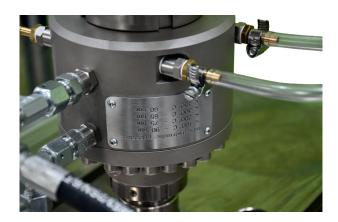
The upper and lower connecting detail (flange) are water-cooled to isolate the grips from the machine (load cell)
