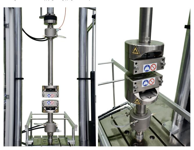
The chamber should have the removable wedge option (U-plugs) in order the chamber can be installed after the grips are installed.
