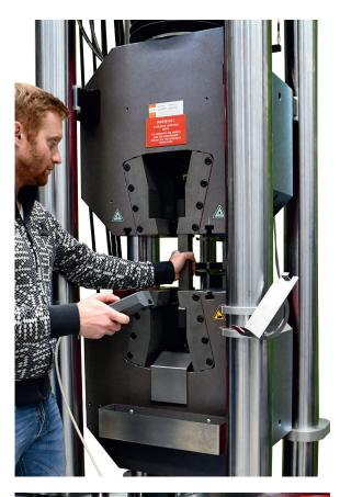
They are the preferred gripping solution for many customers, testing a wide range of specimens and materials including rebars, metallic bars and sheet metals
