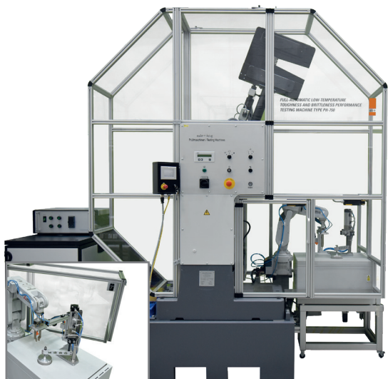
750 Joule instrumented impact tester for temperature range -180°C to +300°C
