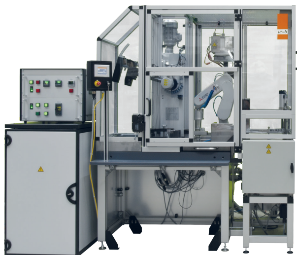
50 Joule instrumented impact tester for temperature range -180°C to +900°C
