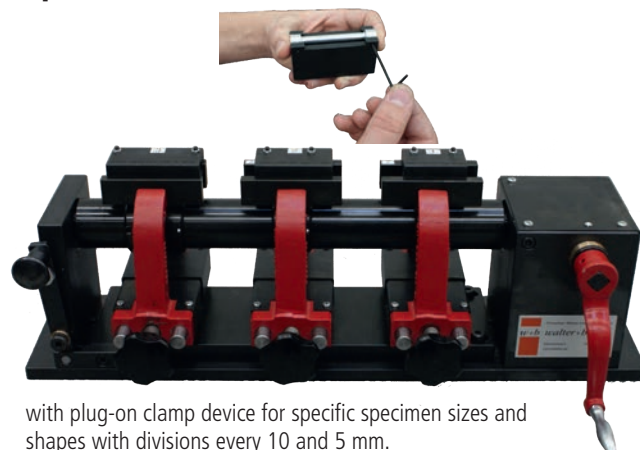
Type TA 200 - 10 / 5 - S Type TA 300 - 10 / 5 - S with 2 clamping devices with divisions every 10 and 5 mm
