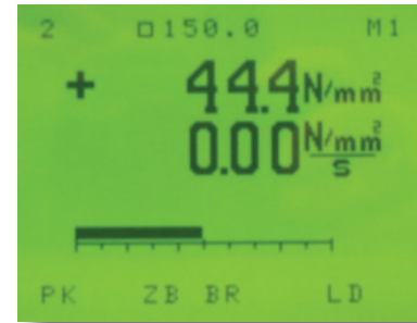
Testing of Cubes Example: Determination of the Compressive Strength of Cubes 150 mm.
