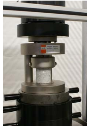
Compression Tests on Small Carrots
