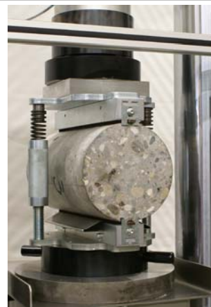
Tensile Splitting Tests on Cylinders Ø 150 or 160 mm
