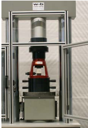
Compression Tests on Half - Cement Prisms
