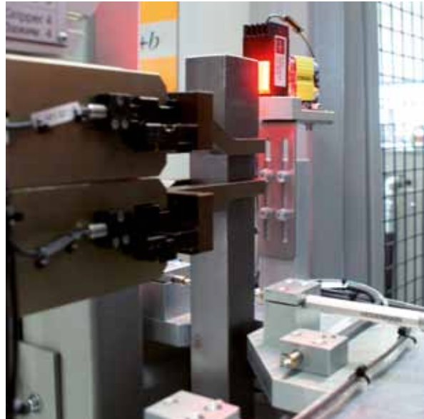
Barcode reader and cross sectional measurement
