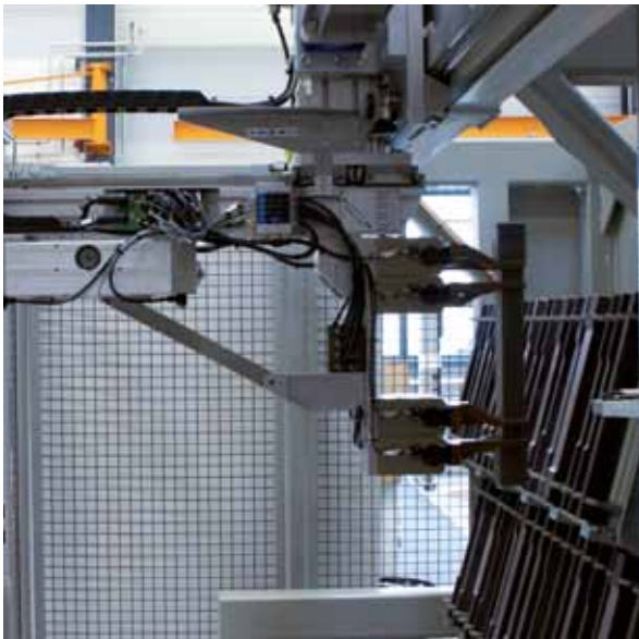
Automatic sample handling out of the magazine
