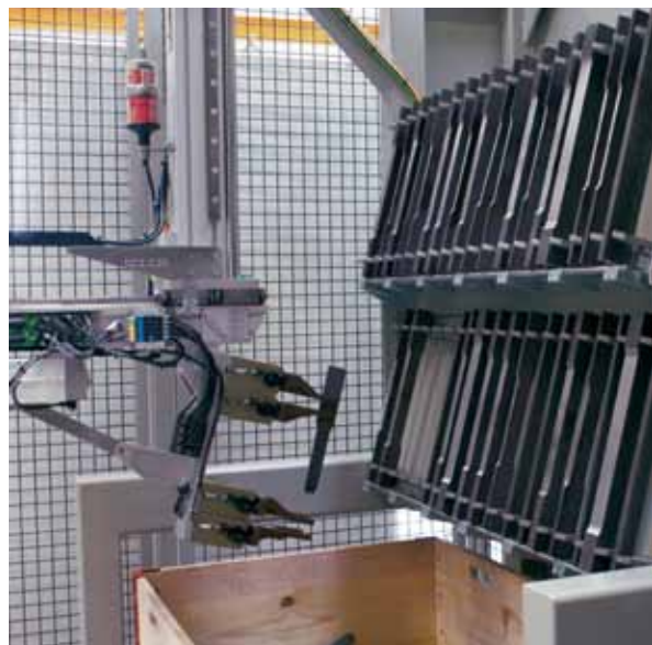
Dropping of broken sample into disposal box
