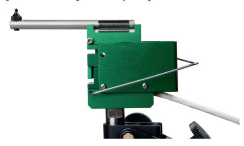
Deflection is measured with a single arm with an attached spherical contact tip, similar to those on a dial indicator. The magnetic base furnished with the gage can be mounted to the desired reference surface, whether flat or round. The tip can then be positioned to measure the deformation encountered during the test. The magnetic base can only be used for low and standard temperature testing.
