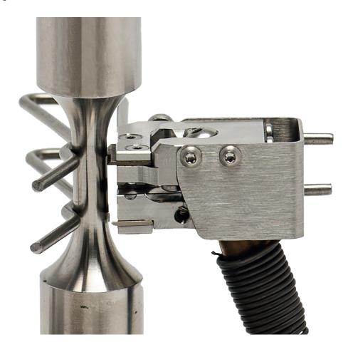
The extensometer come standard with a freestanding sensor conditioner unit providing a electric calibration 0-10 V signal output with exceptionally low noise that can be connected to the strain channel of the controller of the testing system. This conditioner system provides a number of functional enhancements, including high speed digital output, built in calibration and tare functions, analogue and digital filters, and more.
