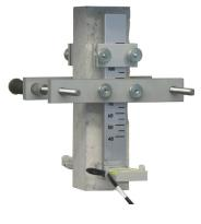
This model measures axial strain on opposite sides of the test specimen with independent outputs making the BD 25/50 suitable for the determination of the Young's modulus on concrete in accordance with EN 12390-13, ASTM C469, ISO 6784 and DIN 1048-5.
