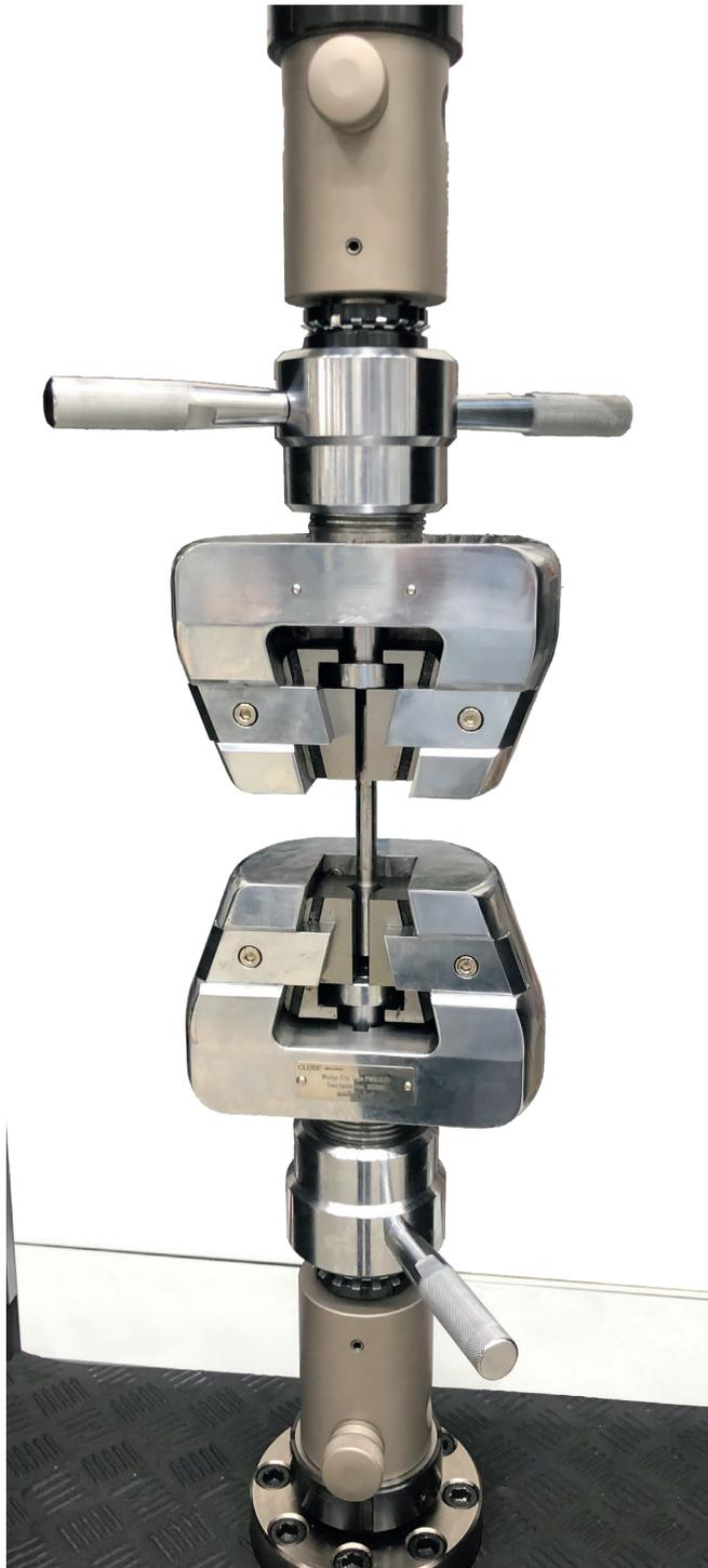
These self-tightening 300 kN grips provide proportional gripping force increase that minimize specimen slippage without the need for pneumatic or hydraulic actuation. A low initial gripping force is applied perpendicular to the flat or round specimen via the handle. The open front design makes specimen loading and changing of the inserts quick and easy.
