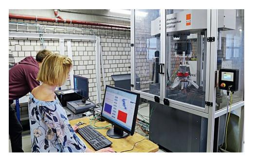
These systems integrate reliable w+b servo-controlled hydraulic actuation with high-resolution & high-speed digital closed loop controls, a broad portfolio of complement accessories and comprehensive Dion7 application software packages making these systems the suitable across the full spectrum of static and dynamic testing including compression, flexural / bending, tension environmental testing application with our related accessories and others.
