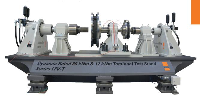
This high torque fatigue rated test systems is used for testing of torsional flexible rubber couplings that compensates radial, axial and angular shaft displacements of the connected machinery. The torque is transmitted by elements loaded in shear. These couplings are available with different torsional stiffnesses and damping factors to satisfy the torsional vibration behaviour of the drive system.
