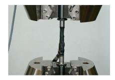
We offer the alignment verification based on ASTM E1012 or ISO 7500-1.
