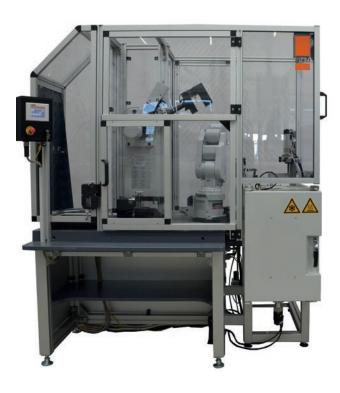
This robotic test system is designed for sub-size metallic samples to perform Charpy Impact Tests according to ISO 148-1, EN 10045, ASTM E23 and instrumented tests in accordance ISO 14556 and ASTM E2298-15 in the temperature range from -180°C to +300°C.
