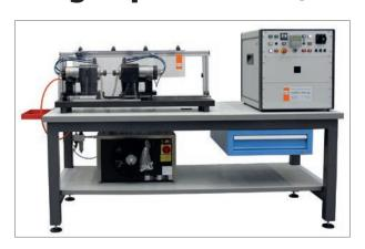
Specially designed for applying of constant rotating load on standard specimen. In accordance with,
