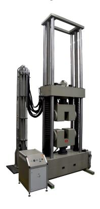
This test system is designed for static testing of round and flat specimens, pillars, columns, beams, carriers made from Carbon, Concrete, Steel as well as Composite Materials. An additional, dynamic rated, servohydraulic actuator
