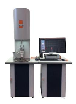
The LFV-E series electrodynamic testing machines provide highly accurate force and motion measurement and closedloop control in combination with our latest ultra-high-speed high resolution Control System PCS8000 with a closed-loop rate of 14.4 kHz and 24 Bit resolution. Tests can be performed in the full frequency
