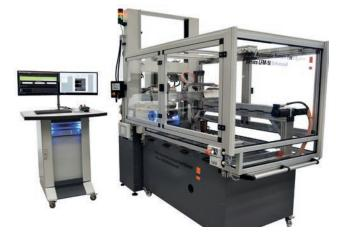
The samples dimensions (width and thickness) are measured in the cross-section measuring device as part of the test cycle.
