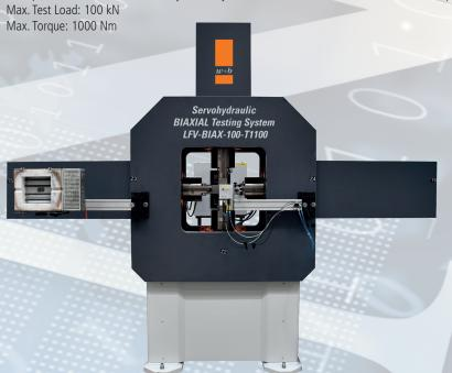
With integrated hydraulic grips, pullpush rods for tests in combination with environmental chamber and pull-push rods for tests in high temperature furnace.
