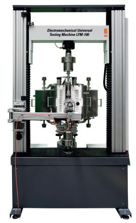
The test duration mainly depends on test specification that dictates the specimen heating rate and holding / soak time. Additionally one also needs time to cool down the furnace and specimen with pull-rod before one can remove the tested specimen from the furnace. With such wait times the throughput with one furnace is limited to few specimens per workday.
