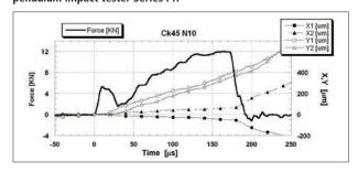
Xi COD Yi Deflection with pendulum impact tester Series PH
