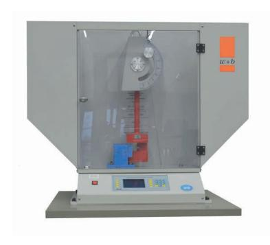
Standard features include advanced dedicated microprocessor control, Touch membrane Alpha / Numeric keypad for data entry, LCD display for sequence logic menu auto prompt selection, Yes / no mode selector, RS232 output with data transfer lead, Specview "Scada" software to allow PC control of Tester and real-time viewing of results, Selfcalibration proce-
