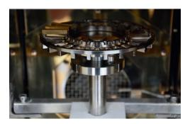
desired temperature (each sample can have individual temperature), and after the soaking time past, tested within the described 5 seconds since removal from the chamber. The test data are transmitted automatically to customers HOST system.
