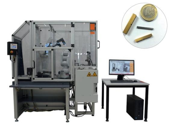
The typical system configuration includes the barcode reader, the sample conditioning chamber, the handling robot, **DION7IMPACT** software package and connection to customer HOST system for data transmission.
