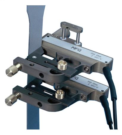
MFQ-H models are equipped with easy exchangeable, fixed BO -stops for fixed initial width of the specimen. The stoppers are easy and quick to change without any tools.
