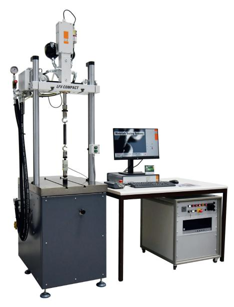
These LFV Compact Series represents ergonomically and space saving test systems ideal for characterizing the static and dynamic properties of materials and components at force capacities up to 10 kN.
